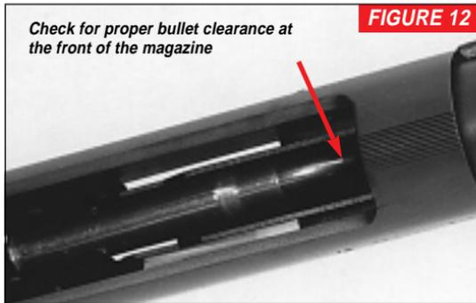
base is seated against the rear of the magazine and that the bullet points have proper clearance at the front of the magazine (See Figure 12).
