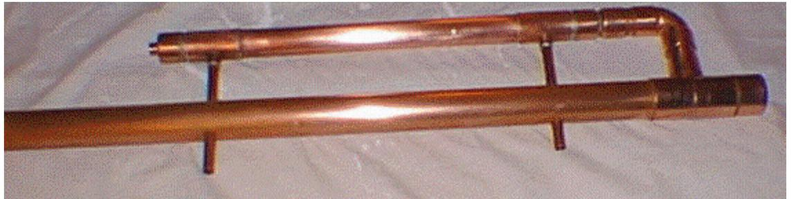
Make sure everything fits OK and aligns well. When you’re satisfied, remove the cooling tubes and condenser. Clean up and solder the 1 ½” elbow and nipples to the column tee. Finally, re-install the cooling pipes to the condenser to assure its alignment, and solder the remaining joints.
