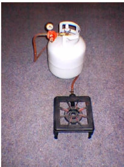
A gas heat source will also react much more quickly to control changes than electric, and is capable of producing far more heat than electrical household circuits can supply.
