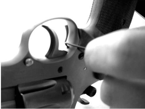
Adjusting the trigger stop screw
