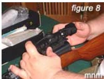
7) The scope came with the rings already attached, so I loosened them and then set the scope in the notches in the mount.
