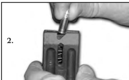
3. When the follower has been depressed, pivot the cartridge so that the rim is under the lips and push the cartridge fully to the rear of the magazine.
