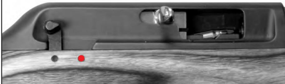
Bolt forward, round chambered, safety off. Ready To Fire.
