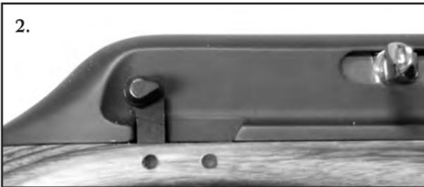
2. Slide the manual thumb safety rearward into the "ON" position.
