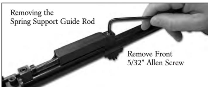
5. To remove the spring support guide rod from the barrel/receiver assembly, back out (or remove completely) the spring guide rod locking screws with a 5/32" Allen wrench.
