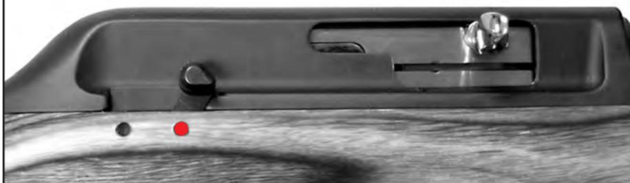
Bolt traveling back, empty case being ejected.
