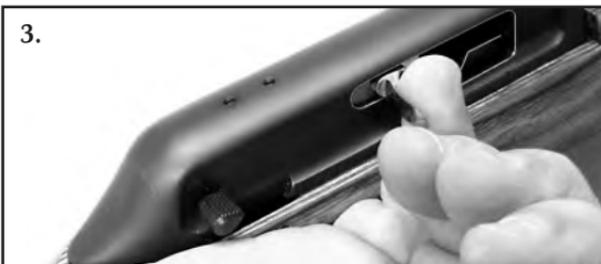
3. Pull back on the bolt handle. (with an empty magazine inserted, the bolt will remain locked in the rearward position)
