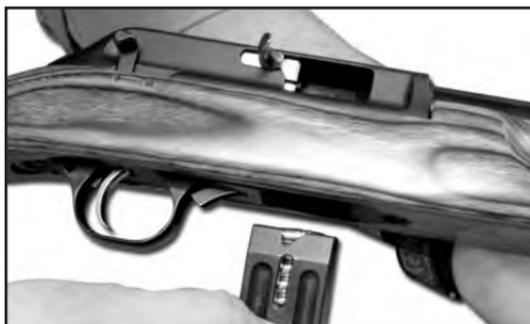
The bolt of your Model R55 can be in 2 positions. It can be locked in the rearward position, held by the bolt stop, or it can be fully forward against the chamber of the barrel.
