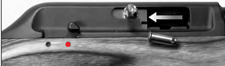
Bolt locked rearward by bolt stop, magazine empty - safety has been manually returned to the "ON" position.
