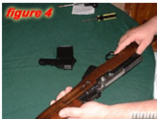
Next came the installation of the 10 round magazine. I tried installing it on my Chinese SKS and found it did not fit right correctly just off the bat. The instructions state - *"The SKS rifles were made by different companies in China. They are not all exactly the same. As with the 10 rd Box, each clip must be fitted to the rifle."*
