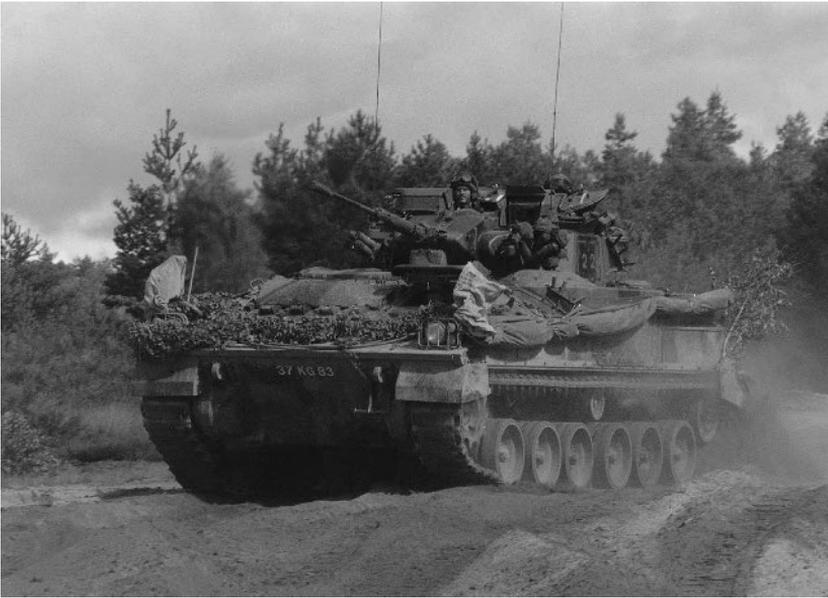
1.3 Warrior armoured fighting vehicle (AFV) utilising Al-Zn-Mg alloys. Courtesy of Alvis Vehicles.
