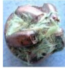
Image of the projectile on a vest of Kevlar      Detail of the end after an impact on a vest of kevlar
