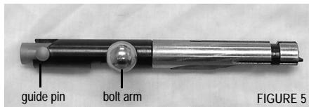
2. Hold the bolt so the firing pin is located top center. With the trigger pulled, slide the bolt into the rear of the receiver.
