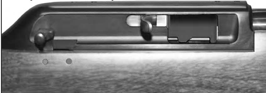
Bolt locked rearward by bolt stop, magazine empty - safety has been manually returned to the "ON" position.
