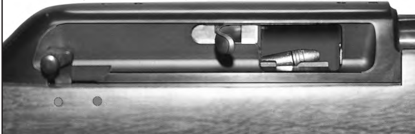
Bolt forward, round chambered, safety off. Ready To Fire.
