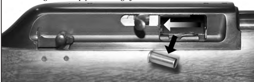
Bolt locked rearward by bolt stop, magazine empty - safety has been manually returned to the "ON" position.
