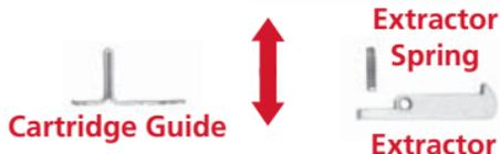
4. Remove cartridge guide, by removing end from hole and pulling wire from slot. Pull wire down to remove.
