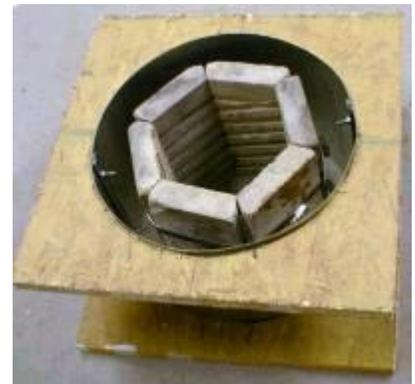
Now you are ready to ram in the refractory around the firebrick. Be careful not to ram it too tightly, or the insulating properties may be defeated. I like to use the a rubber hammer handle to tamp this in, as the weight of the hammer itself is just about right to sufficiently pack the refractory. **Level off and smoothly trowel the refractory at the top of the heating chamber.**
