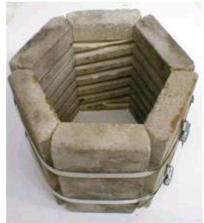
Refer to the drawing on the next page (*Inside Brick Layout*) for accurate detail of how the bricks should fit together. Your measurements may vary somewhat depending on how close you were able to get the bevels cut, but this is no problem. If the bricks don't fit together satisfactorily, you can always cut the bevels more.
