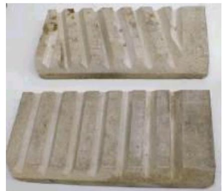
straight bricks with one setting before adjusting to the next groove. It helps to make the grooves line up perfectly when each groove is cut the same on all bricks!
