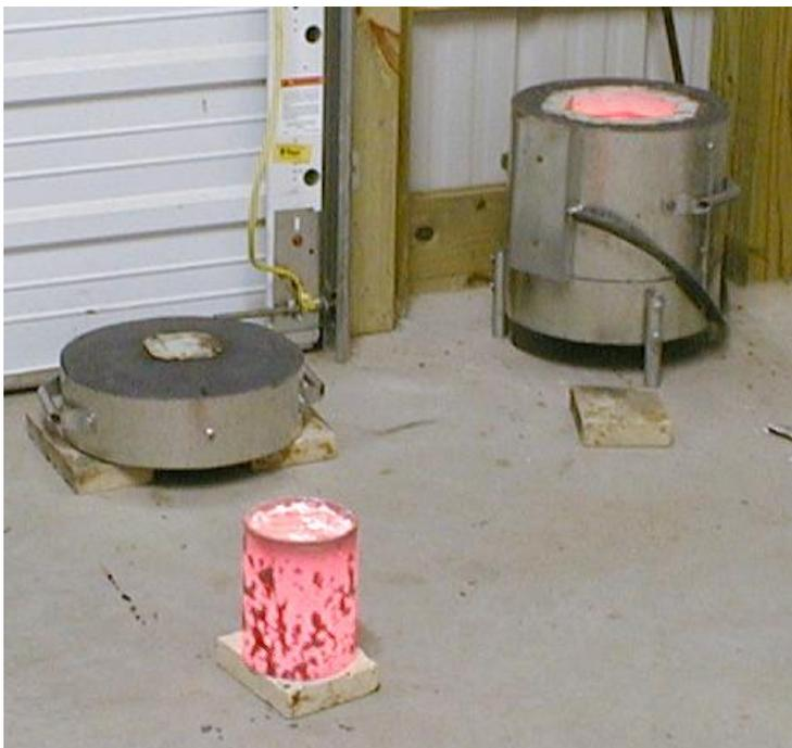
Note the use of firebrick to set hot objects on. You must do this to avoid damage to the floor of your workshop. Setting a red-hot crucible directly on a concrete floor could result in an explosion! It is also a good idea to put an inch or two of sand on the floor under your furnace to curb a leak of molten metal should it occur.
